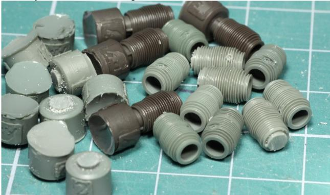
Place the cylinders in the holes in the crankcase - only one correct position is possible. For best results use a two-component epoxy glue to have enough time for the correct alignment of the elements.
