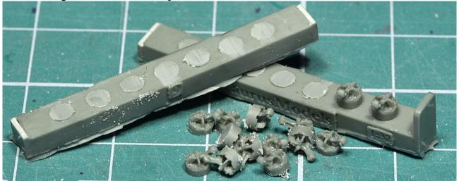
Next put the heads into the holes in cylinders. Use two-component glue, in order to
