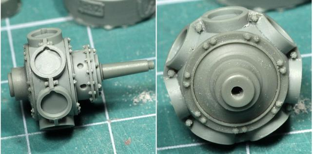
Additional hole at the back of part 12 can be helpful for further assembly - the match or skewer can be used for holding.
