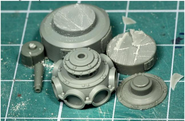
Connect the crankcase elements (2) and (12) using a two-component epoxy glue (this
