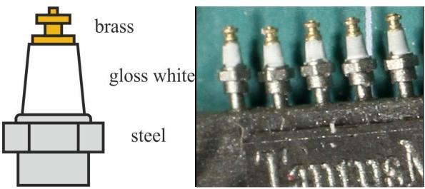
Paint each elements on steel color (I used Gunze Super Iron SM02) instead of back plate of the engine (backelite color) and tappets bushes (part 8) - brass color (I used Gunze Super Gold SM03).
