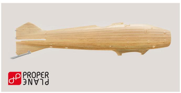
5. Trim the 'finger joint' decals and apply around the fuselage from the front to the back. Note that decals use transparent film to achive a realistic, 'blended' finish on your model.
