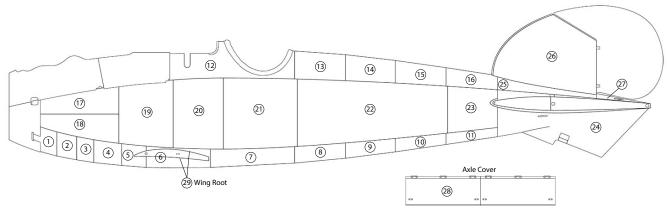
2. Apply the fuselage decals in the numbered sequence shown on the sheet. We recommend that you start from the bottom panels, then top ones, leaving the side panels for last.
