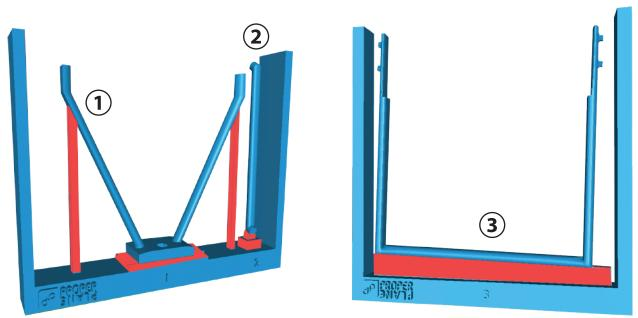
Before starting the assembly all the parts should've be removed from the frames and print supports. Print supports are marked with red. Cut the parts off with a knife with sharp blades.
