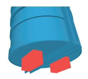
Remove the red marked supports from the barrel part.
